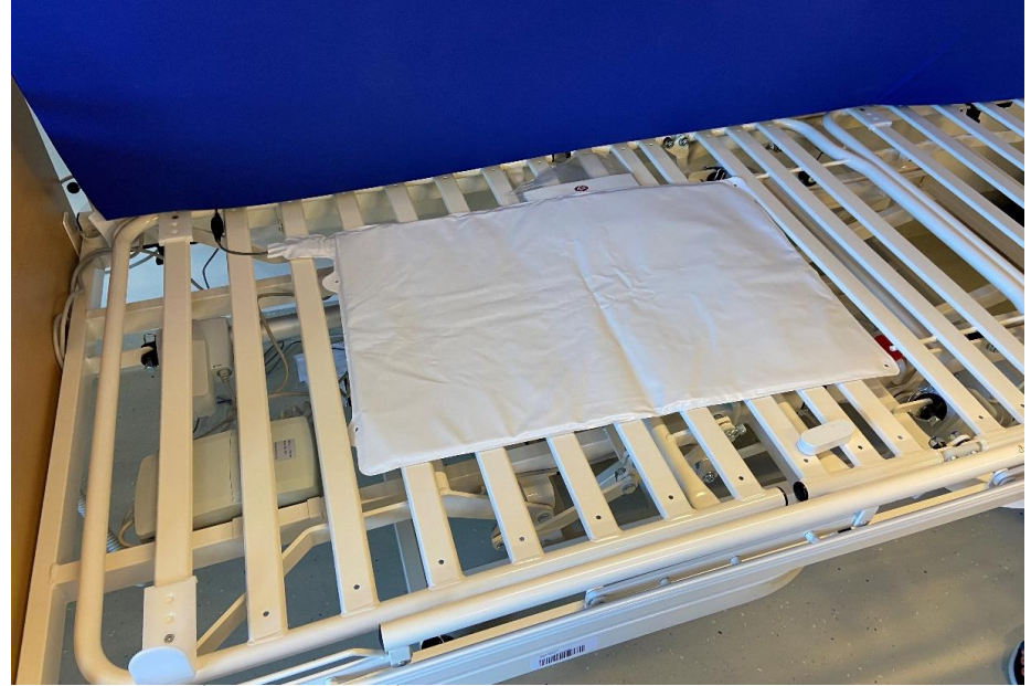
The bed sensor installed at the bed frame underneath the mattress
